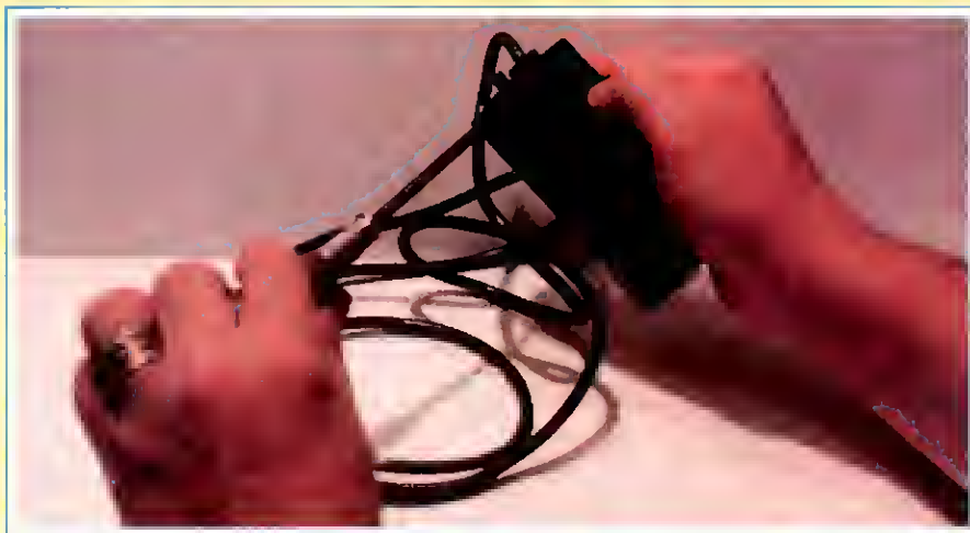
FIGURE 1: Using a Phillips screwdriver, remove the screw holding the RF modulator box together. Then slide off the box's cover.
